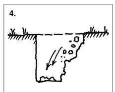
The sides collapse, reducing the amount of water that can be collected and allowing surface water to get into the well from the top.
