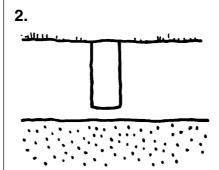
They are not deep enough, so water is inaccessible in dry weather when the groundwater level is low.
